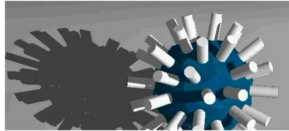
**Figure 1** A possible realization or model of a nano-, or pico-lander. The sensors can be found in the prickly-like cylinders protruding from the central sphere which have the support leg function also [2].,
