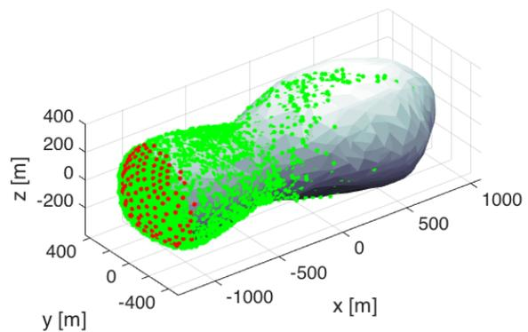
Figure 4: Landing sites of the particle ejected from the tips. The ejection velocity is 0.15 m/s.
