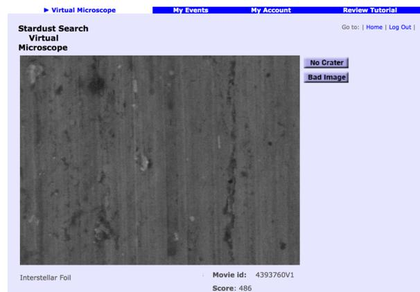
Fig. 1: A typical field of view on the foils search VM. The width of the field of view is  $41\mu\text{m}$ .
