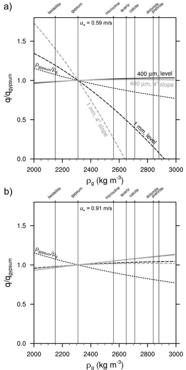
**Figure 1.** The saltation mass flux  $q$  of 400 μm and 1 mm grains relative to gypsum grains of the same size calculated at a)  $u_* = 0.59$  and b)  $0.91$  m/s. The dotted line shows the creep mass flux relative to gypsum grains. At  $u_* = 0.59$  m/s, saltation of 1 mm grains segregates them by density far more efficiently than creep; however, this relation does not hold in much stronger winds.
