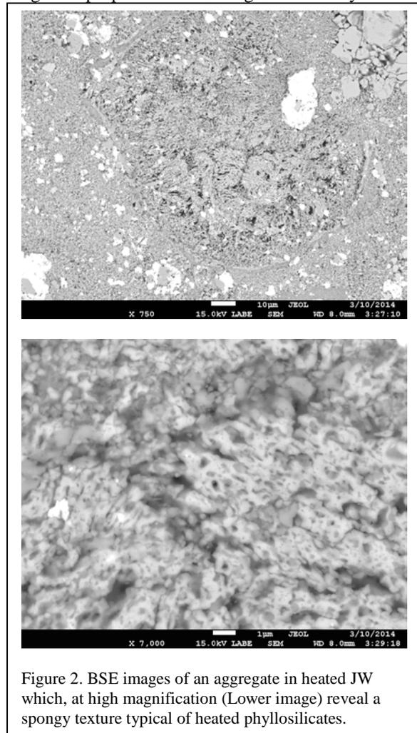
Figure 2. BSE images of an aggregate in heated JW which, at high magnification (Lower image) reveal a spongy texture typical of heated phyllosilicates.
