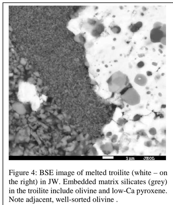
Figure 4: BSE image of melted troilite (white – on the right) in JW. Embedded matrix silicates (grey) in the troilite include olivine and low-Ca pyroxene. Note adjacent, well-sorted olivine .
