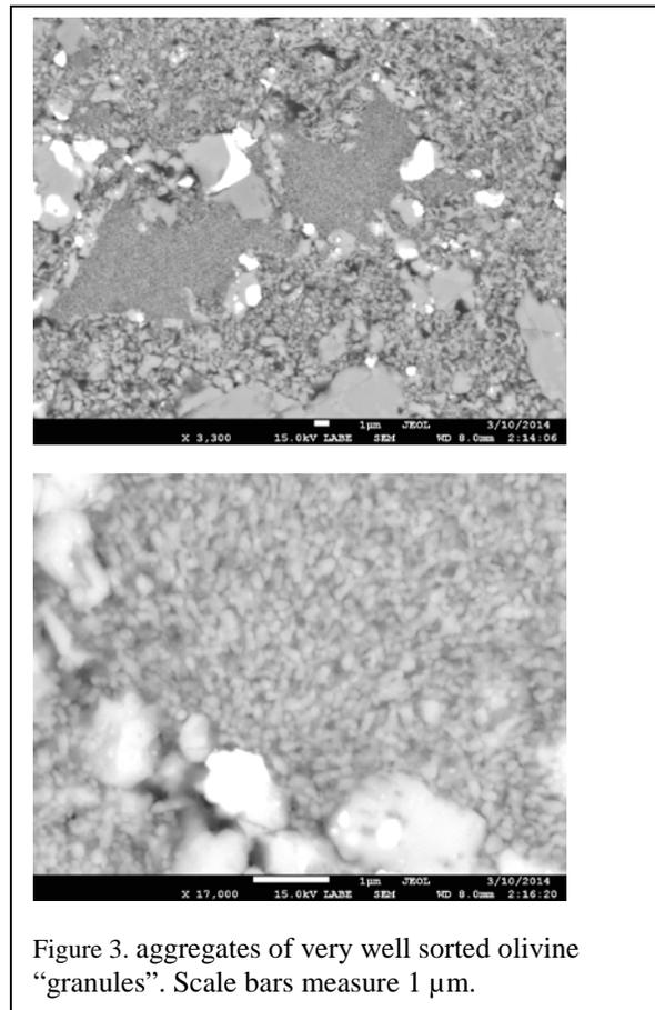
Figure 3. aggregates of very well sorted olivine “granules”. Scale bars measure 1 µm.
