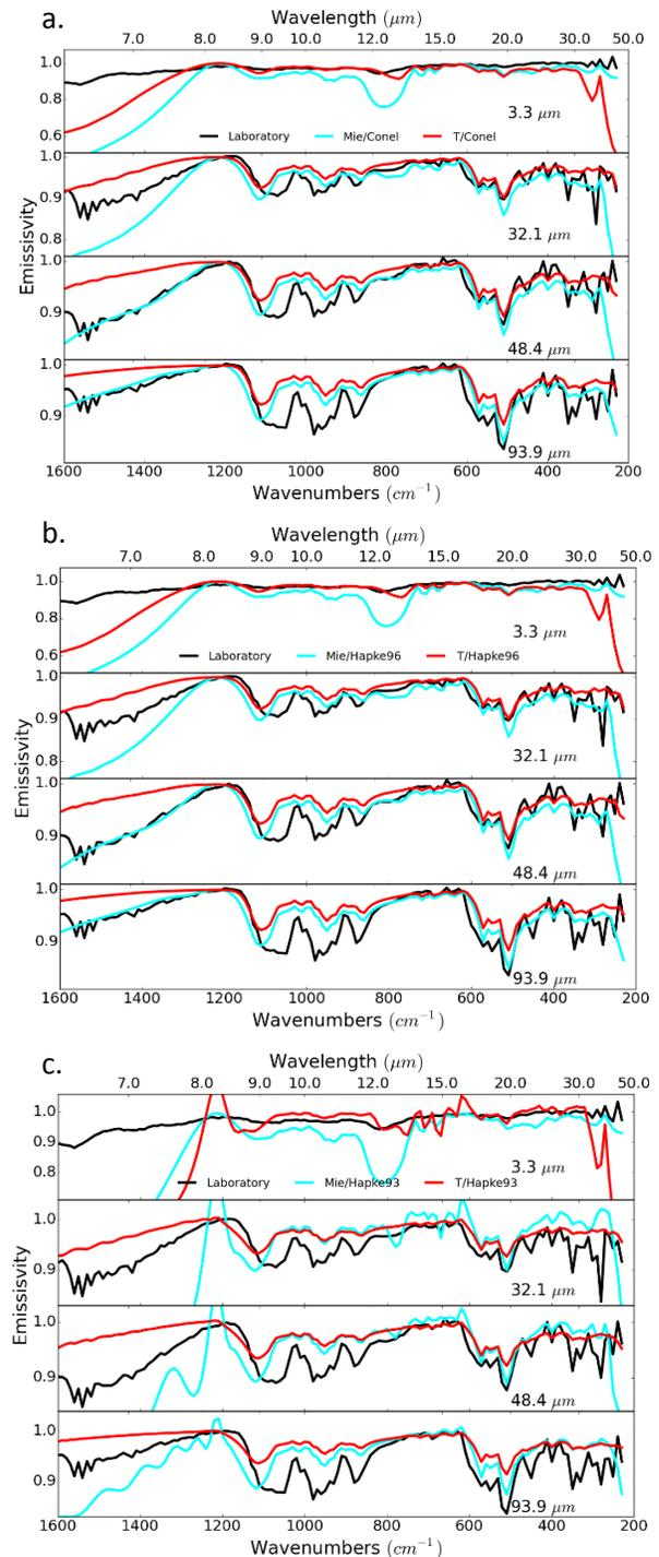
Figure 1. Computational and laboratory emissivity spectra of enstatite particulates. Models used in computation are T-matrix and Mie models coupled with radiative transfer models of a. Conel (1969), b. Hapke (1993), and c. Hapke (1996). Each plot contains spectra for 4 different size fractions where means of each size range, measured in laser diffractometry, are indicated.
