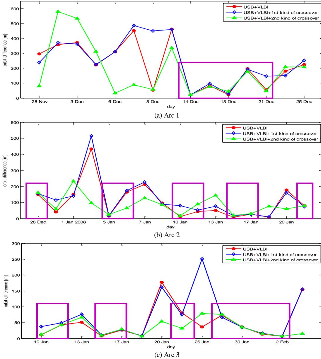
**Fig.2** RMS of total orbit overlap differences for CE-1 (tracking data include ranging measurement and VLBI measurement in purple rectangle. Otherwise, only ranging measurement is including.)
