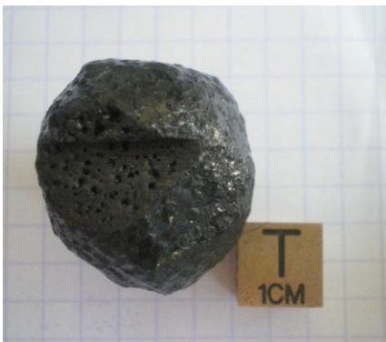
Figure 1. The Vic specimen (once cut in the upper corner). It has a bright outer layer that reminds a fusion crust, and its interior exhibits mm-sized bubbles.
