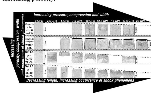
Fig. 2. Thin section scans of the four experimental series cut parallel to the propagation direction of the shock front and through the center
