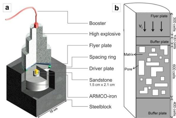
Fig. 1. (a) Experimental set-up for the shock recovery experiments. (b) Illustration of the meso-scale model set-up including the sample with a defined number of randomly distributed pores.
