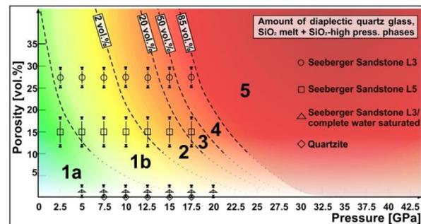
Fig. 3. Pressure calibration of shock stages 1a to 5 for porous sandstone versus porosity. The isolines of the amounts of diaplectic quartz glass, SiO<sub>2</sub> high pressure phases, and SiO<sub>2</sub> glass represent the limits between shock stages 1b to 5. The boundary between shock stages 1a and 1b is defined by the complete closure of pore space. The arrow lines at each datapoint represent the range of porosity for the individual targets of the shock recovery experiments.
