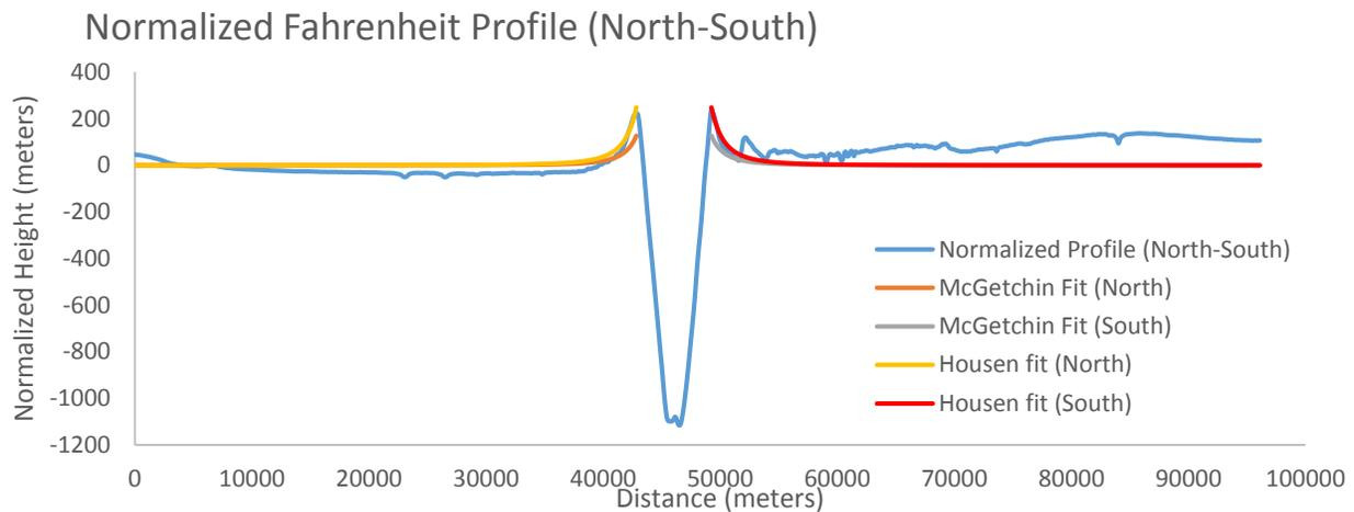
Figure 1 - A normalized topographic profile of Fahrenheit, a simple, 6-km diameter crater located within Mare Crisium (13.1N, 61.7E). Both the McGetchin et al. and Housen et al. models are applied to a north-south cross section view of the crater. The Housen et al. model also shows a near-perfect fit for the crater, with the exception of preexisting (i.e., non-crater) topography.
