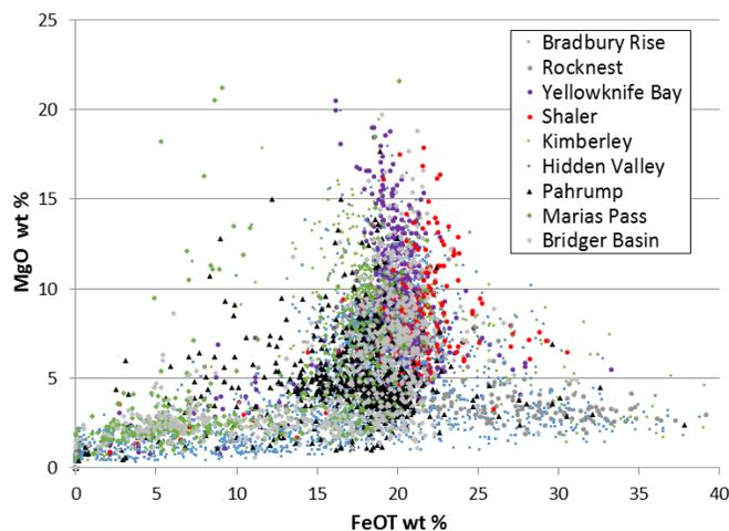
Fig. 3. FeOT vs. MgO abundances. Yellowknife Bay shows some of the highest MgO due to enrichments along ridges that are likely diagenetic features [20]. Rocknest targets show the highest Fe values along with low Mg [12]. Some Pahrump targets enriched in Mg but low in Fe are diagenetic sulfate features.
