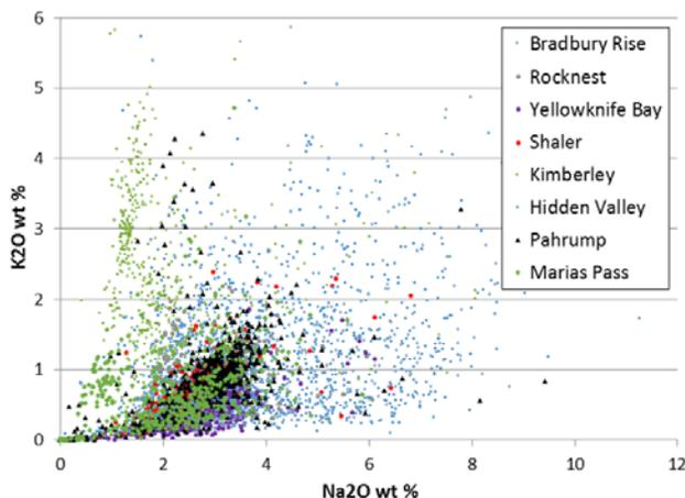
Fig. 4. Na<sub>2</sub>O vs K<sub>2</sub>O abundances. Bradbury Rise points spread to high alkali values reflecting significant feldspar inputs. Kimberley shows distinctively high K, while some Marias Pass points have the same K/Na ratio. Bridger Basin data (not shown) has some of the lowest K/Na ratios.
