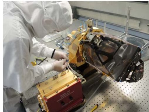
Figure 3. The CaSSIS instrument on the bench (with the senior electronics engineer for scale). The electronics box is to the left. The camera rotation unit is to the right. The telescope is the mostly black structure cantilevered off the golden structure which includes the rotation drive.
