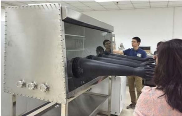
Fig. 2 Glovebox equipment. this figure shows the first step in establishing the nitrogen environment in glovebox. Sample selection, grinding and cutting were performed in this environment. Polished sections preparation was conducted in the atmosphere environment, the use of selected debris and original powder samples were made into the required polished section.
