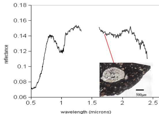
Fig.2. Spectrum of chondrule rim grain (x141y23). The
