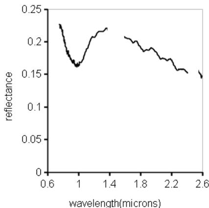
Fig.4. Pixel spectrum of olivine (x109y37). The spectrum is dominated by features near  $1\ \mu\text{m}$ . The other spectral features are related to water absorption. Data in  $1.4$  and  $2.5\ \mu\text{m}$  regions have been removed because of overlapping with instrumental artifacts.
