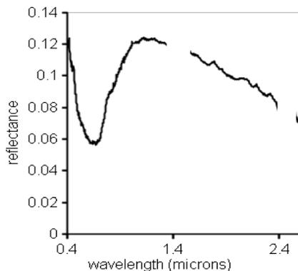
Fig.5. Pixel spectrum of sulfide grain (x109y37), probably MgS [5]. Data in  $1.4$  and  $2.5\ \mu\text{m}$  regions have been removed because of overlapping with instrumental artifacts.
