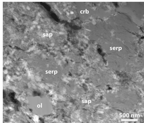
Figure 1: HAADF TEM image of a typical phyllosilicate-dominated region of the microclast; serp: serpentine, sap: saponite, crb: carbonate, ol: olivine.
