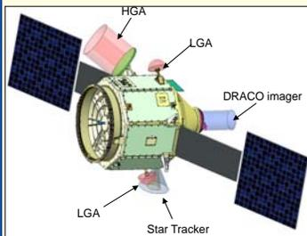
The DART payload is one instrument, a high resolution imager derived from New Horizons LORRI
