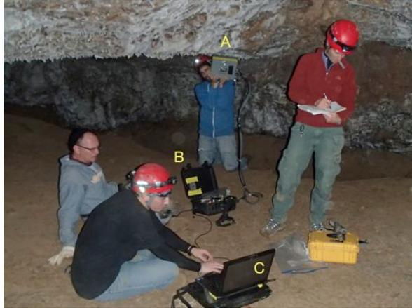
**Figure 2:** PASA operating in Fort Stanton Cave. The steel box containing the optical head (A), the electronics box (B), and the ruggedized laptop (C) are labeled. Here, we measured the IR spectrum of a gypsum star shown in Figure 3. Photo credit: Wayne Walker.
