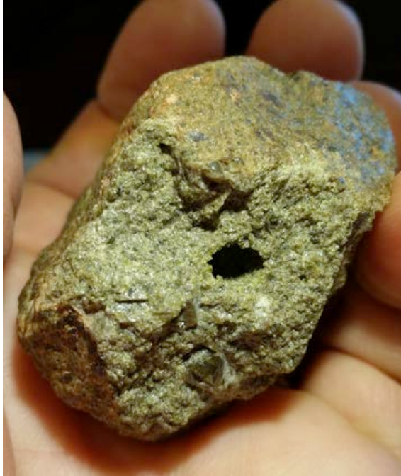
Fig. 1. Hand sample, the NWA 8535 main mass, broken surface reveals green olivine crystals and prominent cavity (dark shadow).
