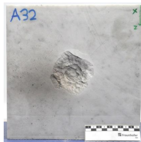
Fig. 1: Experimental impact crater formed in a Carrara marble target. The crater were formed by a 4 mm aluminum projectile at \sim 7 km/s. Target is 25x25x25 cm.
