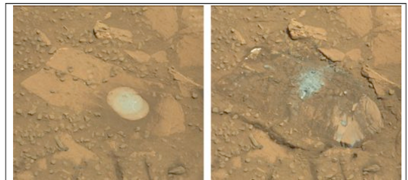
Fig. 2: The Bonanza King site after DRT-ing the rock (left), and after the failed mini-drill hole (right). Notice how the slab has shifted during the mini-drill attempt and appears to be partially depressed into the subsurface material. This resulted in a 'successful' drill failure when rover hardware detected the shift and halted activity before damage could be done to the PADS system. Dirt Removal Tool ellipse is roughly 40 x 60 mm.
