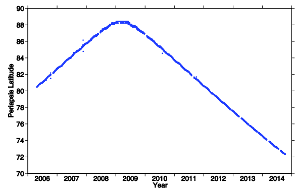
Figure 1. The periapsis of Venus Express has been decreasing in latitude ~3° per year since 2009.
