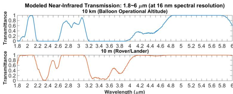
**Fig. 1:** Near-infrared transmission as a function of wavelength at two altitudes above Titan's surface in a model Titan atmosphere. The spectra are sampled to that of VIMS resolution (16 nm) [19]. All methane transmission windows widen considerably at balloon altitudes when compared to those from orbit, and widen even further for a rover/lander (see Fig. 2 for a direct comparison).
