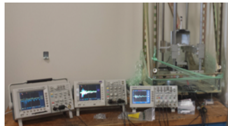
Figure 3. Drop tower setup for typical 9 channel impact data collection. Each PZT is connected to a different channel on one of the three oscilloscopes shown.
