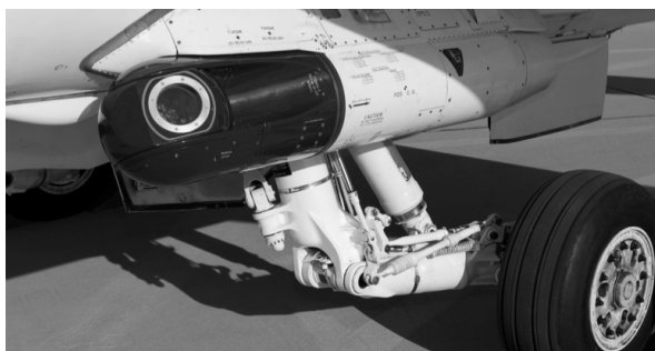
Fig 1: NASA's two seat F/A-18B Hornet, carrying the FLIR pod (under left fuselage) based at the Armstrong Flight Research Center. Backseat observer can in real time control the 11" telescope 8 \mu m camera.
