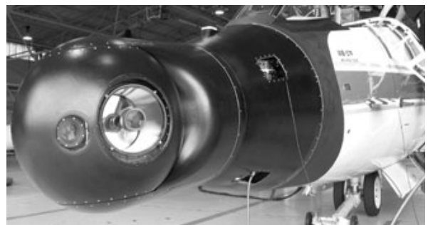
Fig 5: The WB-57F/DyNAMITE telescope mounted on the nose cone. A dichroic allows simultaneous observations at visible and infrared wavelengths.
