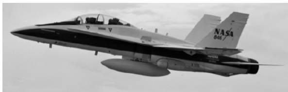
Fig 1: NASA's two seat F/A-18B Hornet, carrying the FLIR pod (under left fuselage) based at the Armstrong Flight Research Center. Backseat observer can in real time control the 11" telescope 8 \mu m camera.
