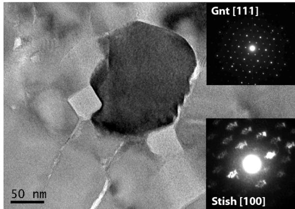
**Figure 1.** TEM image of the shock-vein edge assemblage of majoritic garnet (Gnt) and stishovite. The stishovite tetragonal prisms appear as light-gray square crystals. Phases were identified by SAED (Gnt) and CBED (stish) diffraction patterns.
