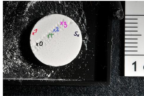
Figure 1: Target pellet of forsterite (synth.) colored numbers correspond to spectra of the same color in Fig. 2.
