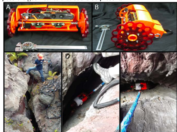
Figure 2 Photos showing VolcanoBot. A, B: Photograph of recently modified VolcanoBot2, a rotary microspine robot, with 12.5 cm diameter wheels and a 25 cm long body. C-E: Field-testing of VolcanoBot1, 20 cm diameter wheels and 35 cm long body. C: Lowering the robot into a volcanic fissure vent at Mauna Ulu. D: Foot for scale with VolcanoBot1 in the fissure. E: VolcanoBot1 beginning to map the fissure. The tether (blue) spans 30 m, and includes two power cables, a data cable, and a mechanical tether.
