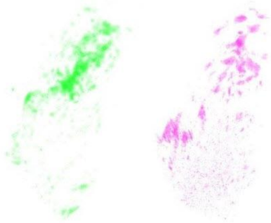
Figure 1. Three dimensional reconstruction of Si-O stretch in silicates (left) and C-H bend in aliphatics (right).
