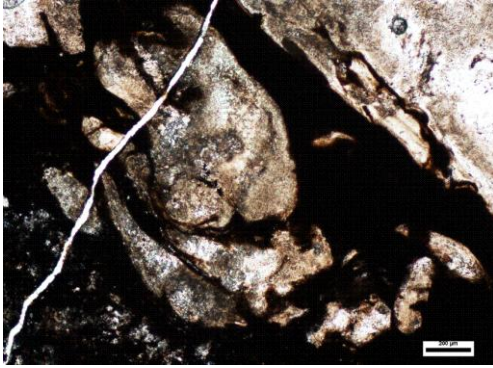
Figure 3. A plagioclase clast within the melt vein of WCIS-14-AR-016 with evident flow textures in plane polarized light.
