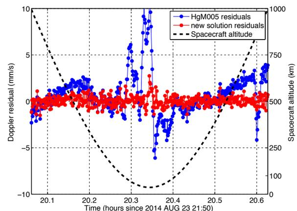
**Figure 2.** Line-of-sight Doppler residuals (in mm/s) relative to the *a priori* field (HgM005,  $l_{\max}=50$ ) and our new solution ( $l_{\max}=75$ ). Large gravity-related signals at low spacecraft altitude (black dashed curve) were not previously observed.
