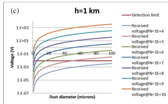
**Figure 1.** Expected peak output voltage of detector versus dust diameter when the flight altitude is (a) 20 km (home position), (b) 5 km, and (c) 1 km. Detection limit (about 9 mV) of the detector is also shown.
