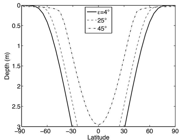
Figure 2: Model-predicted depth-to-ice after 4.5 Ga of desiccation for obliquities  $\epsilon$  of  $4^\circ$  (best estimate of current value),  $25^\circ$ , and  $45^\circ$ . In all cases, there is shallow ice in the polar regions. The depths are the same on both hemispheres, because the rotation axis is assumed to precess due to perturbations by other bodies. Not taken into account is devolatilization by impact gardening.
