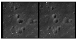
Figure 2: Left image shows an uncontrolled mosaic seam, right image shows the controlled mosaic seam.
