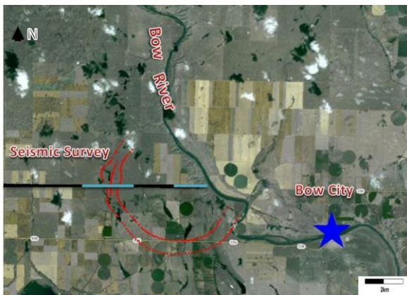
Figure2. Map of the seismic survey. Blue lines are the high resolution lines line1 (left) and line2 (right). Black line shows the location of the earlier study in figure1. The red curve shows the estimated rim faults (Source: Google Map).
