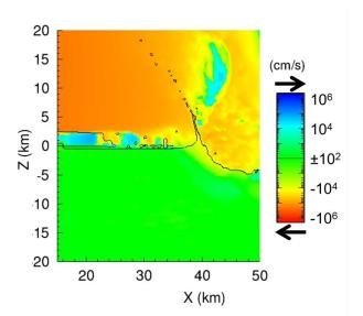
Figure 2 - CTH x-velocity plot of a 3D calculation at 18 s into the calculation. Plot shows the impact of a 1.5 km diameter dunite projectile into a basaltic target overlain by 500 m of porous water-ice. The projectile impacted from right to left at 45° and 12 km/s. Note the color and direction legend on the right. Blast-wind velocities reach at least 100 m/s. Vortices begin forming downrange at the surface with tornadic intensity prior to arrival of ejecta.
