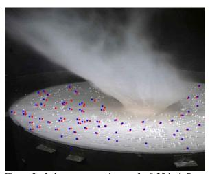
Figure 3 - Laboratory experiment of a 0.25 inch Pyrex projectile impacting dolomite at  $45^{\circ}$  (from the right) and approximately 5 km/s. Red dots indicate the initial position of some of the Styrofoam pearl tracers. Blue dots indicate the position of the tracers at 1935 µs into the impact. Impact vapor expansion interacting with the ambient atmosphere mobilizes the tracers to meter per second velocities.
