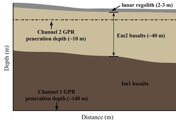
**Fig. 2.** A schematic diagram shows a three-layer subsurface structure model at the landing site.
