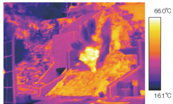
Fig. 4: Infrared video image of the crater formation process.
