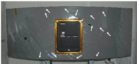
Fig. 1. The WFPC2 radiator shield wrapped in Llumalloy sheeting at the Johnson Space Center (NASA-JSC), locations of the large craters indicated by arrows.
