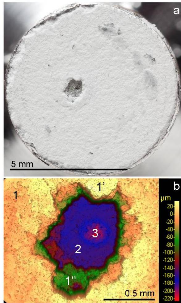
Fig. 2. WFPC2 sample 121: a) optical image; and b) DEM, showing: 1 paint external surface; 1'' partially exfoliated paint; 2 exposed surface of aluminium alloy; 3 compound crater pits in the surface of alloy.
