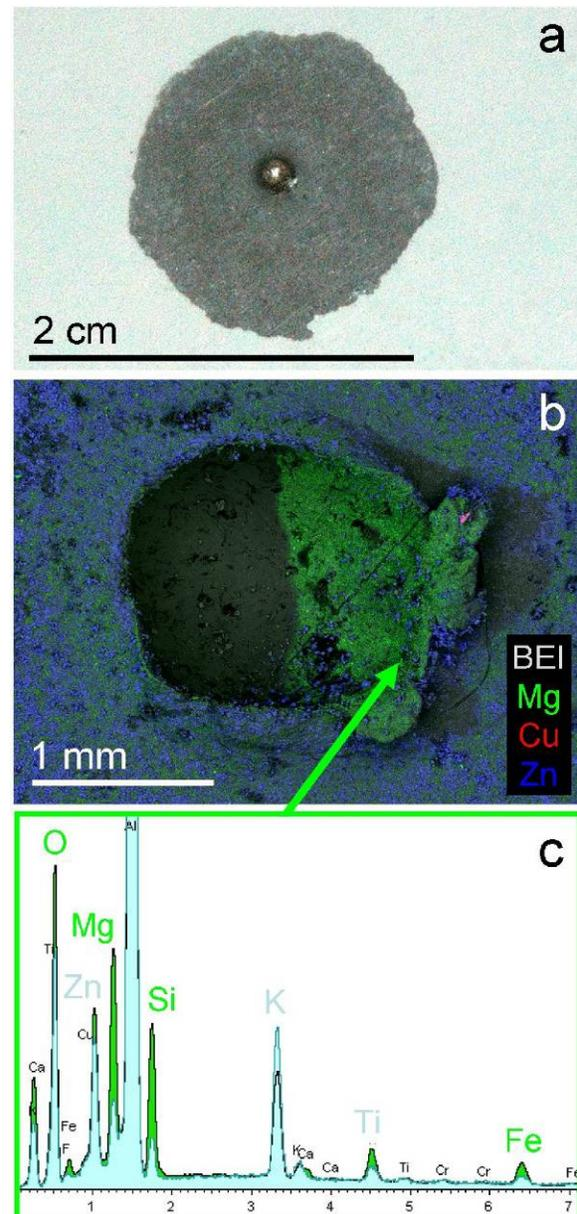
Fig. 4. WFPC2-424: a) optical image; b) EDX maps c) Mg-, Fe-silicate fragment, probably shocked olivine.
