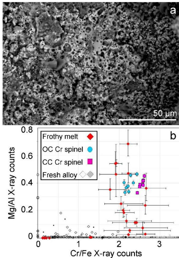
Fig. 3. WFPC2 sample 121: a) BEI of frothy impact melt outside compound pits; b) plot of melt composition in Mg/Al versus Cr/Fe X-ray counts compared to ordinary and carbonaceous chondrite Cr-rich spinels.
