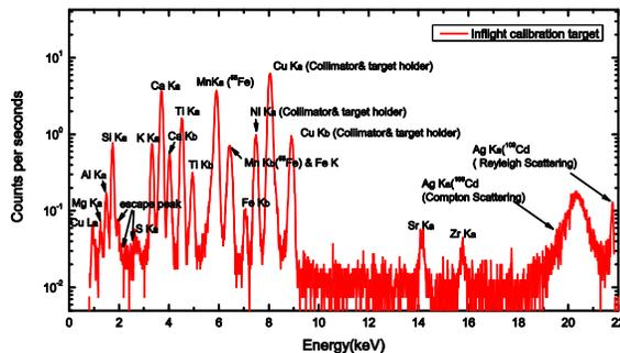
Figure 4 Spectrum of calibration target
