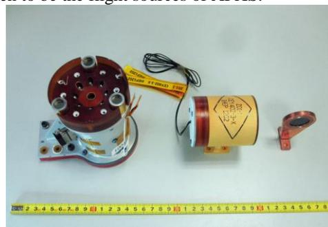
Figure 3 APXS components: sensor head, RHU and in-flight calibration target (from left to right)
