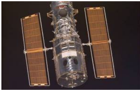
Fig. 1. a) HST seen from orbiter Discovery during service mission 3A (STS-103) in 1999. The 2.2 m wide WFPC2 radiator surface is covered in white ZOT paint.
