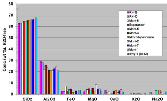
Fig. 5. The aluminosilicate end-member (red bars, after extrapolated silica is subtracted) has Si and Al in the common range for montmorillonites, with appropriately low values for other elements.
