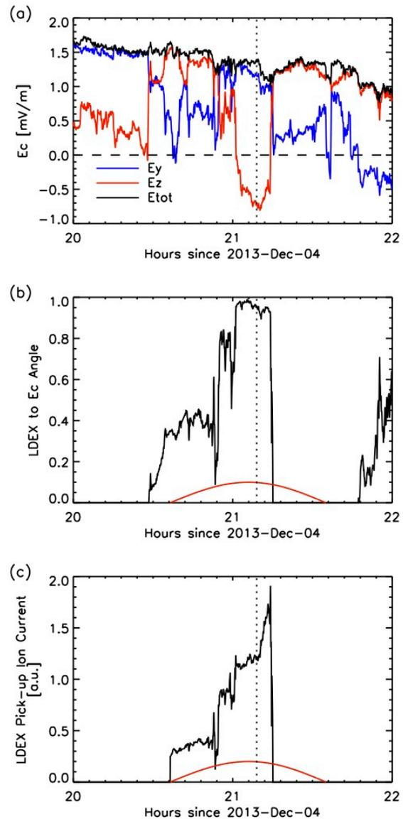
**Figure 3:** (a) The convection electric field components (colored lines) and magnitude (black line) as measured by the ARTEMIS spacecraft. (b) The cosine of the angle between the convection electric field and the LDEX instrument boresight. (c) The model-predicted pick-up ion current into the LDEX instrument in arbitrary units for approximately one orbit on December 4, 2013. The red semi-circle denotes the period when LADEE/LDEX was on the lunar dayside.
