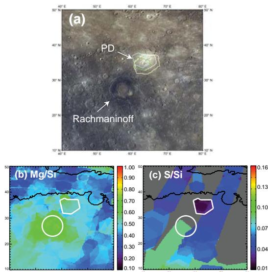
Figure 2. (a) Color image of Mercury for the region surrounding the NE Rachmaninoff impact basin and nearby PD. Polygons indicate outlines of footprints for XRS spectra used in chemical analysis of the PD. (b) Mg/Si and (c) S/Si maps of same region; white circle and polygon indicate Rachmaninoff basin and XRS measurement footprint of PD, respectively. Black lines indicate outlines of northern volcanic plains.
