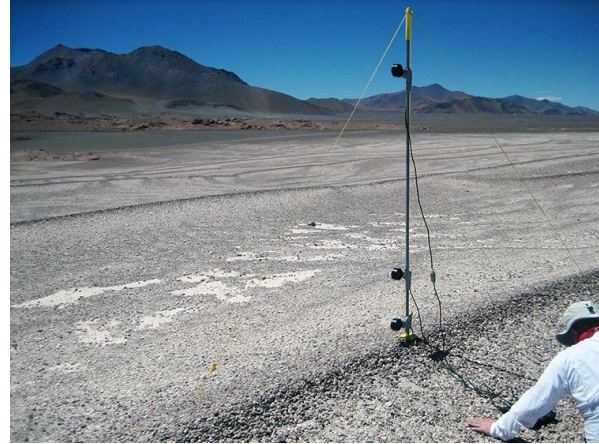
Figure 2. Wind profiling station on crest of megaripple at Campo Purulla [2]; this site showed the strongest form flow effects. (JRZ, 12/6/10).
