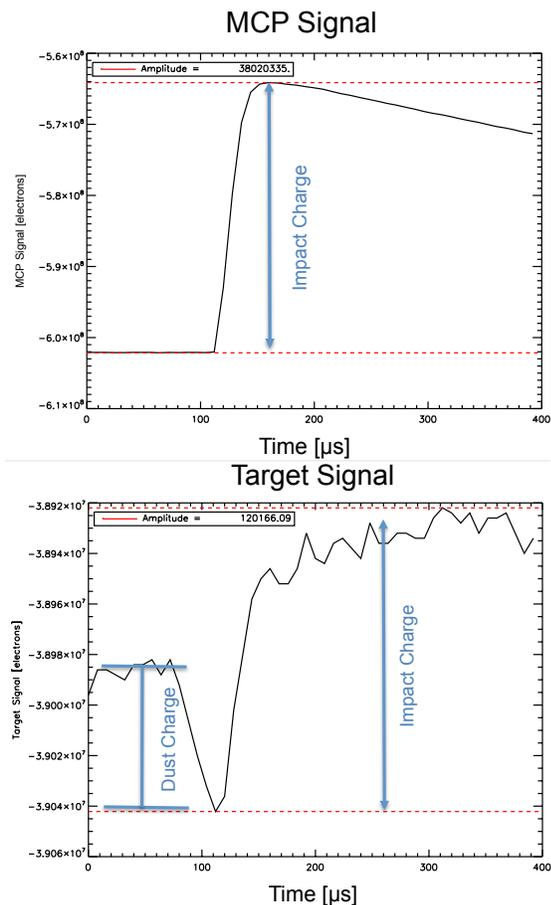
**Figure 3.** Impact waveforms recorded by LDEX at the Colorado dust accelerator of an iron particle with a radius of 1.06  $\mu\text{m}$  and speed of 1.89 km/s. The waveforms are recorded (50 samples with a dt of 8  $\mu\text{s}$ ) and transmitted to ground. At the accelerator the dust particles are highly charged and the target signal also shows the effect of their 'image' charge on the target.
