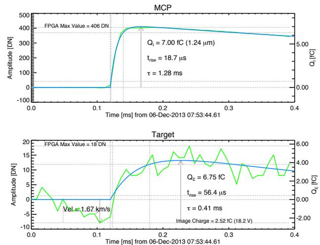
**Figure 4.** Impact recorded in orbit around the Moon on 12/06/2013. Based on preliminary analysis, this particle had a radius of  $\sim 1.2$   $\mu\text{m}$ , and carried a charge of  $\sim 2.5$  fC. The green and blue lines show the recorded waveforms and an analytical fit, respectively.
