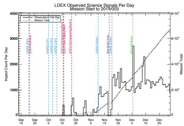
**Figure 2.** Summary of LADEE/LDEX activities through 1/3/2014. The number of recorded events (noise and dust impacts) sharply increased following LADEE orbit lowering maneuvers (OLM). An unusually large burst of events was observed on 11/12/2013, most likely related to the Taurids meteor shower. The following intense period starting 12/13/2013 coincides with the Geminids shower and the landing of Chang'e-3.
