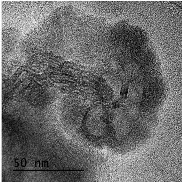
**Figure 2.** Holey onion-like carbon from the polyphase carbon aggregate, HRTEM image.
