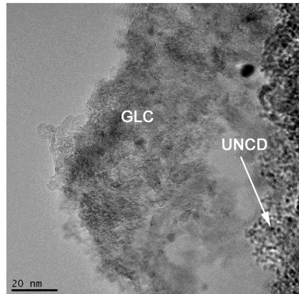
**Figure 1.** Bright field TEM image of polyphase carbon aggregate: glass-like carbon (GLC) and ultrananocrystalline diamond (UNCD).
