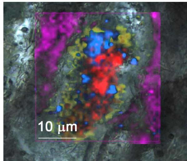
**Figure 1.** Combined optical image of the UHPHT vein impact glass from the Kara meteorite crater in transmitted light with Raman mapping by mineral phases within: red – coesite, yellow – silica glass, violet – aluminosilicate glass, blue – region of the high luminescence (smectite region).
