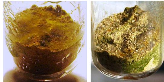
**Fig.1.** (Left) Intensive water sublimation takes place soon after inoculation, cyanobacteria colonize superficial layers of AMG; (Right) After 8 months - Colonially distributed cyanobacteria and Carbonaceous deposits are visible.
