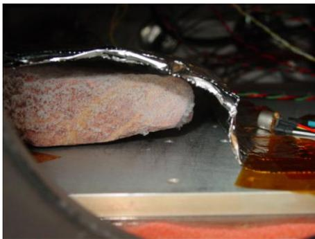
Fig. 1. Frost-covered banded sandstone viewed through external view port on the MSC system.
