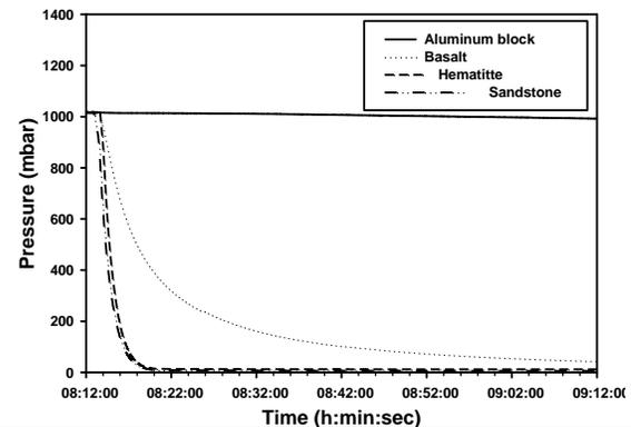
Fig. 2. Rapid degassing of all three rock types occurred between 10 (sandstone and hematite) and 60 (basalt) min.
