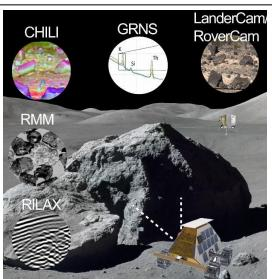
**Figure 1.** The SILICA instrument suite is designed to provide a comprehensive understanding of a landing site's geochemistry, mineralogy, structure, formation, and evolution through time.
